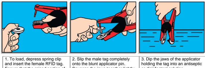
Ensure that the raised portion of the tag, which encloses the transponder chip, is placed in the open portion of the jaws.
